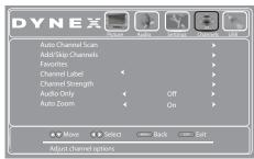
3 Press ▲ or ▼ to highlight Auto Channel Scan, then press ENTER. The CHANNELS-Auto Channel Scan screen opens.
